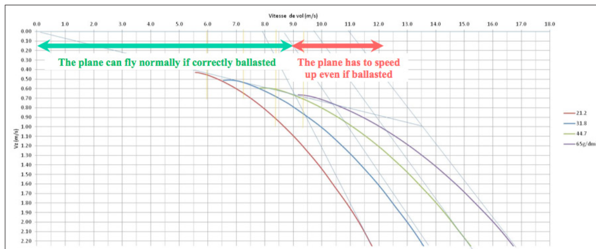
Figure 1: Up to 9m/s wind, a plane can be ballasted as per FAI regulation and flew in a standard way. It is possible to fly at minimum sinking rate... Over 9m/s, this is no more true, and even if fully ballasted (at 75g/dm 2 as allowed), the plane has to speed up to go upwind. This then requires a specific trimming (pitching) for such occasion.
