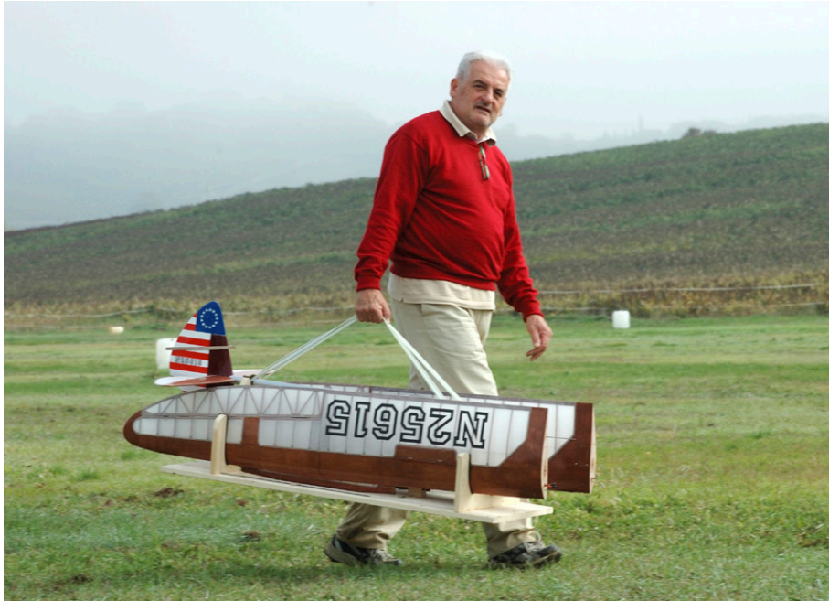
Photo 11: A custom cradle holds all of the parts for transport.
