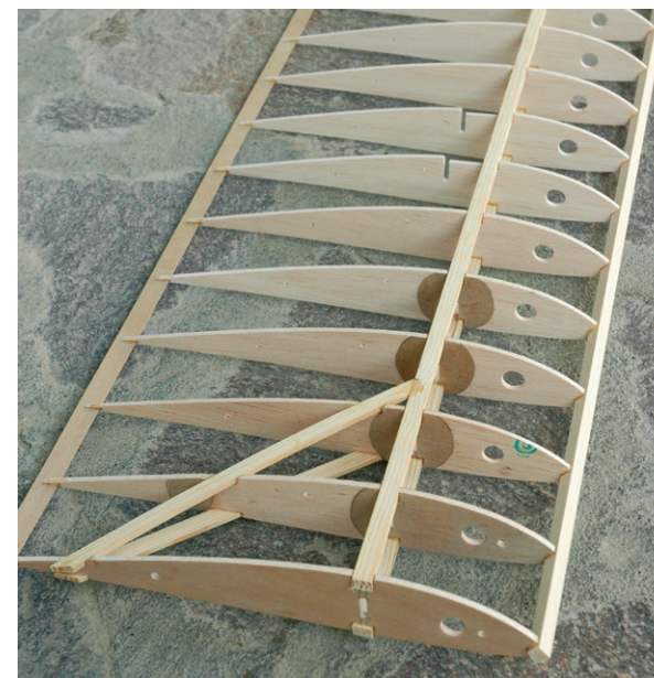
Photo 5: The left wing panel showing spar, ribs and spoiler bay cut-out.
