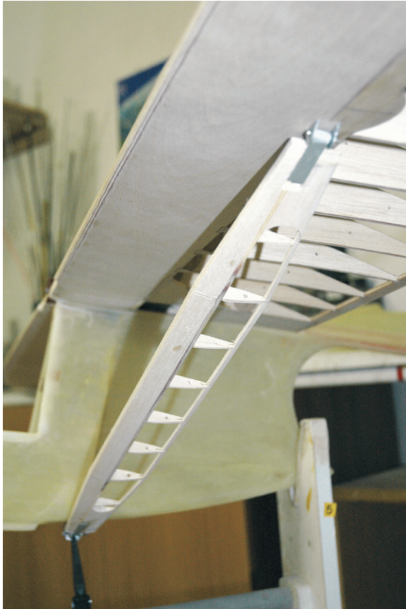
Photo 6: One of the ribbed struts.
