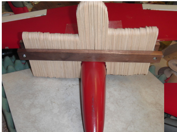
Above: Outside servo tray contour Right: Servo tray contour allowing for fuselage wall thickness
