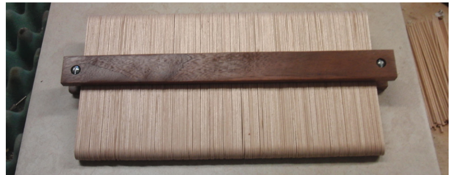
Assembled contour gauge ready to use
