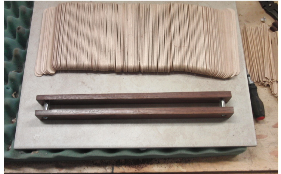
Contour gauge holder with plastic tubing over screws
