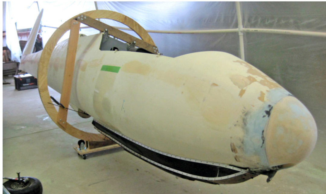
The Ka-2b is shown installed in a wooden ring or "rotisserie" with additional supports made from 2"x4" lumber.
