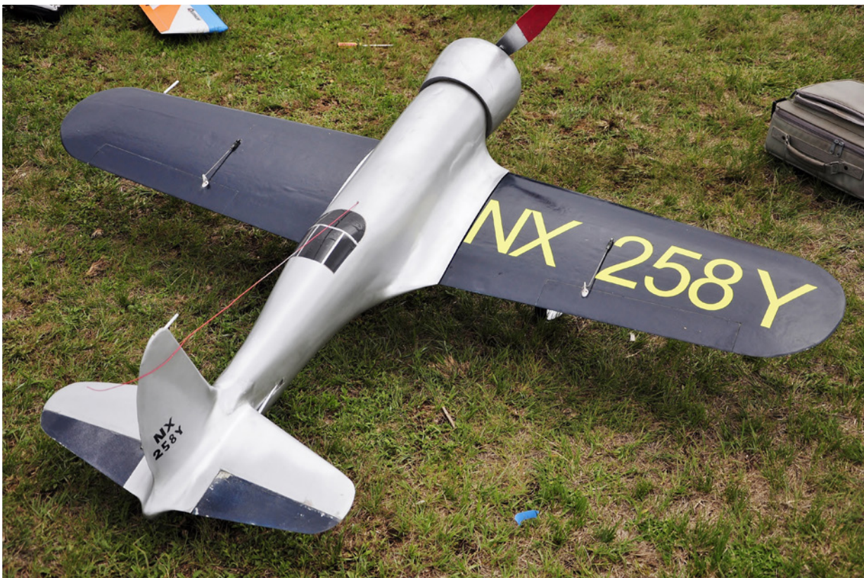
Piet's Hughes H-1 racer. As with his Aero Commander, Piet fabricated a landing gear for this model, removeable for flight.
