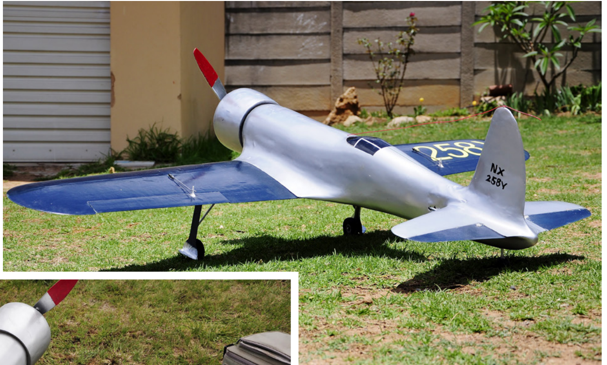
Piet's Hughes H-1 racer. As with his Aero Commander, Piet fabricated a landing gear for this model, removeable for flight.
