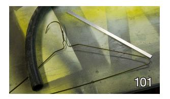
(103) The coat-hanger I bent into a U shape, that'll be inserted into the nose and act as an anchor for the front of the skid. The other hardware will attach the skid to the anchor...
