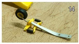
especially if I'm going to aerotow this puppy. (Thanks for the idea there Josh and Gunny). Ideally I'd like a BIG honking wheel in there but I've run into a problem. The carbon fiber bar I ran down the inside of the fuselage is in the way.
