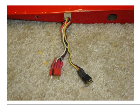
Standard practice with Deans connectors is to use the male part in the wing. When not connected it has no power applied so can't short to other stuff.
