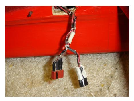
The female Deans connectors are used in the fuselage wiring. The hole in the side is just large enough to pass the connectors. This means I have to use hemostats to feed the wiring and connectors through the holes.
