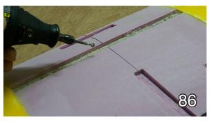
(86) While I had the Dremel tool out I also cleaned out some of that yucky looking Gorilla Glue from the wing-rod slot...
