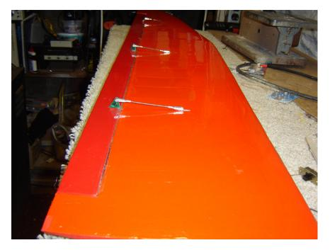
This is the lower surface of the starboard wing panel of the Apache. It has inner and out flaps and also ailerons. The means that there are three servos in each panel. 3-conductor cables are spliced into the wires from each servo and insulated with shrink tubing.
