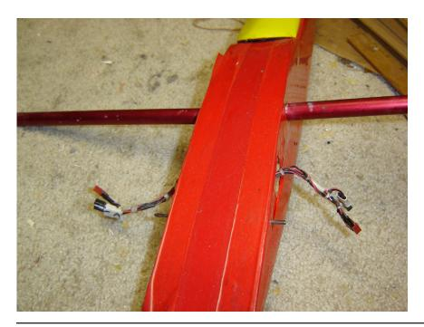
The wiring in the fuselage is brought out from holes just aft of the main wing rod. Since the rudder is controlled using pull-pull cables this wiring was positioned and tied in place to avoid resting on the rudder cables.
