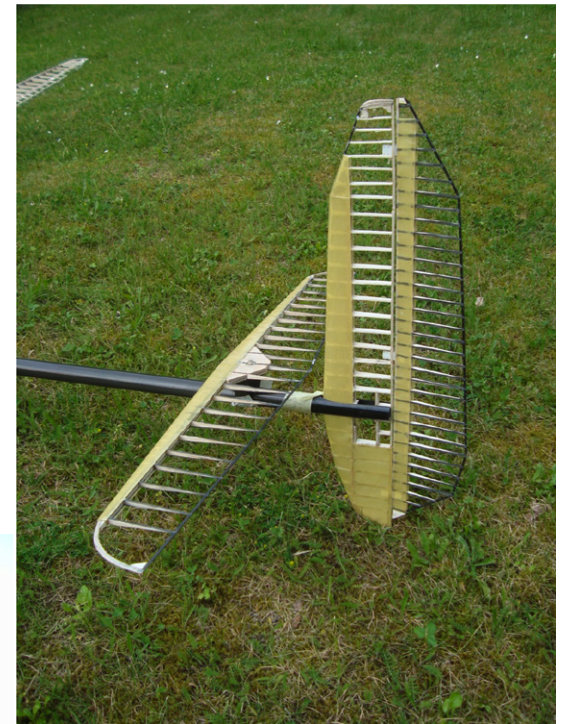
Figure 17a: Vertical fin and rudder and horizontal stabilizer mounted to fuselage before covering.
