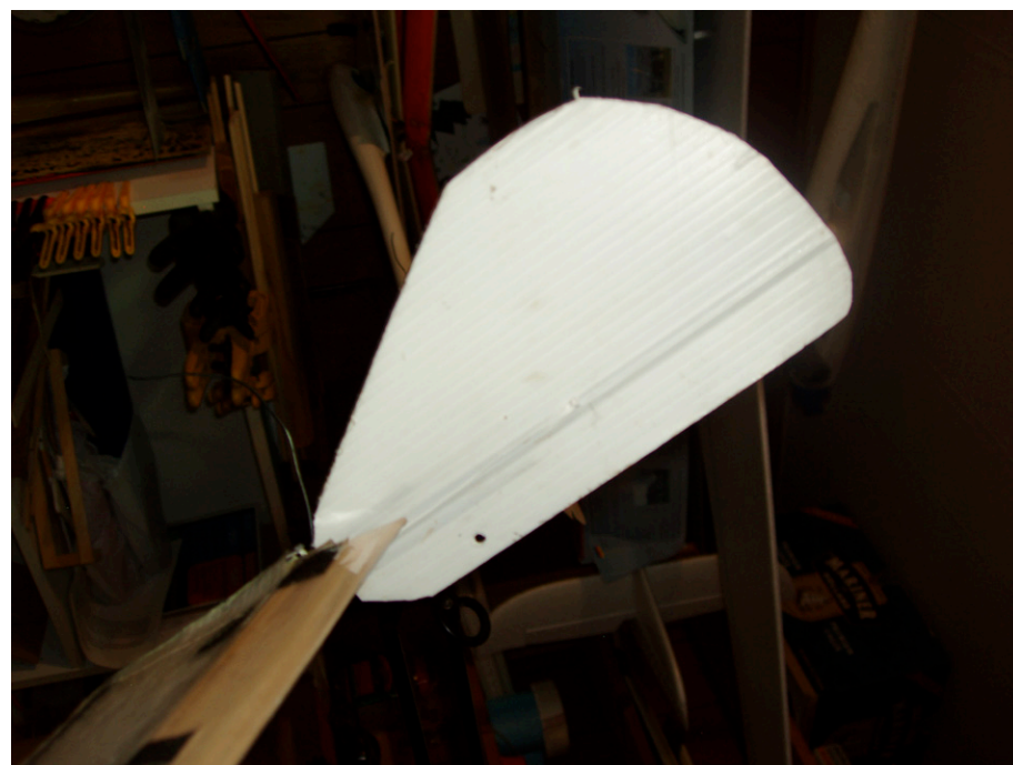
Fin with thicker, tougher, 0.10" spar. The surviving smaller spars still work for vertical alignment
