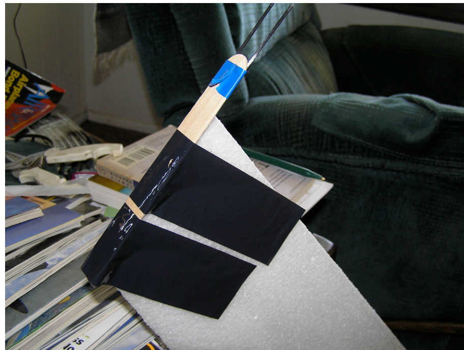
Alignment by tongue depressor
