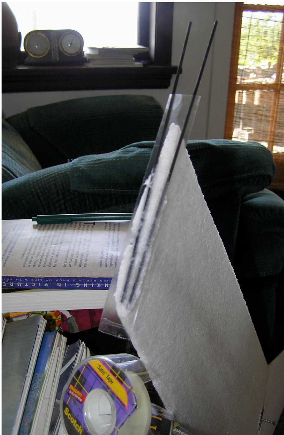
Tape is a mold release
