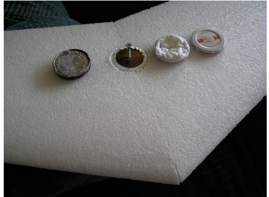
Foaming ballast pit with Gorilla Glue and water
