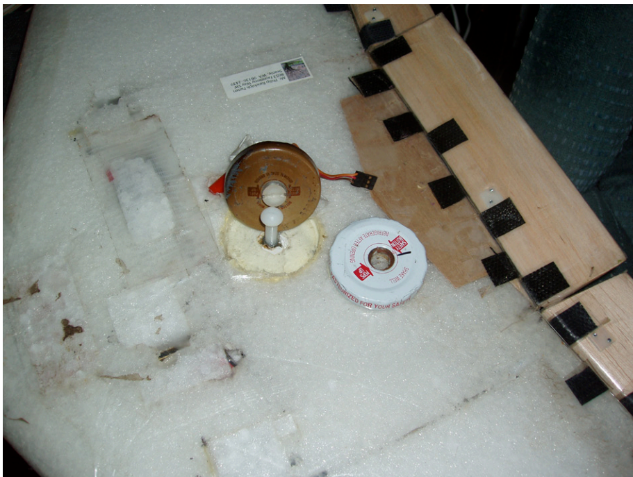
Note countersunk hole for flat- head nylon bolt
