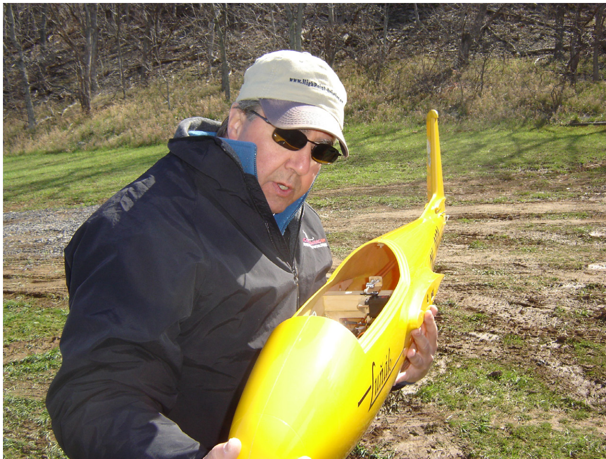
Above: Jim Dolly holds the Lunak fuselage as the elevator controls were checked out. It had two pushrods, one to each elevator half, joined to single ball link at the servo. Pushrod lengths were individually adjustable to set trim.
