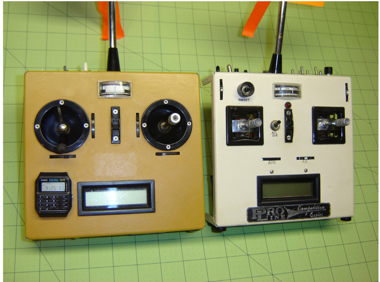
The Kraft/M*2K and the Proline/M*2K are shown. The number of switches and controls of the newer transmitter reflect how experience has led me to develop the design. While the LCD display is a gem, I still like the warm, fuzzy feeling of seeing the iron needle RF meter above the on/off switch.
