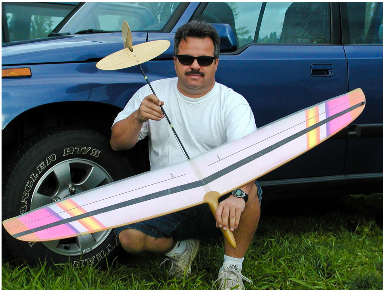
Bruce Kimbel with an early Encore DLG. Bruce airbrushed water-based acrylic paint on the foam core before bagging to get the color trim. Photo by Phil Pearson
