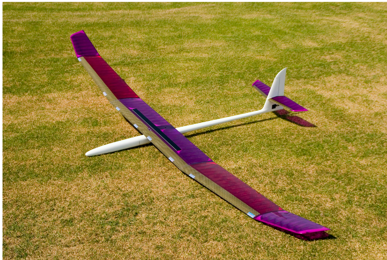
Mark Nankivil's Soprano RES — rudder, elevator, and a single spoiler (the black rectangle just behind the carbon/Kevlar wing leading edge D-tube). Photo by Mark Nankivil
