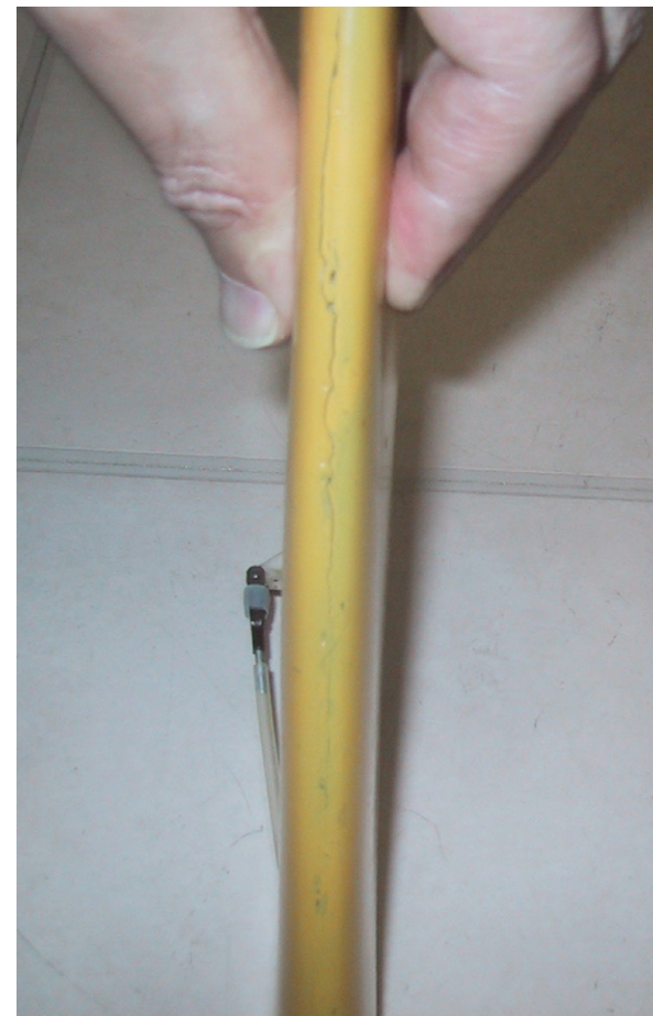
Illustration 7: Under pressure the vertical fin reveals its little secret: it's cracked from top to bottom. This is the result of the vertical fin bending and vibrating sideways on hard landings.
