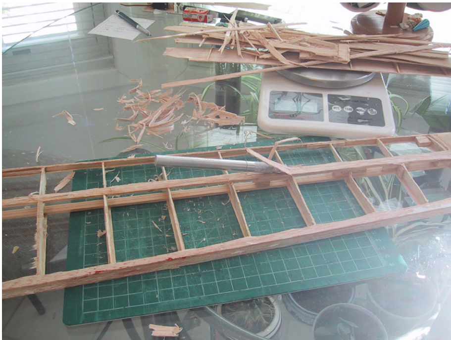
Above left: Illustration 11: The old wood has been sanded down so much, presumably during repairs and recovering, that it had to be built up and sanded flush with the new sheeting in places like these rib caps and around the servo wells.
