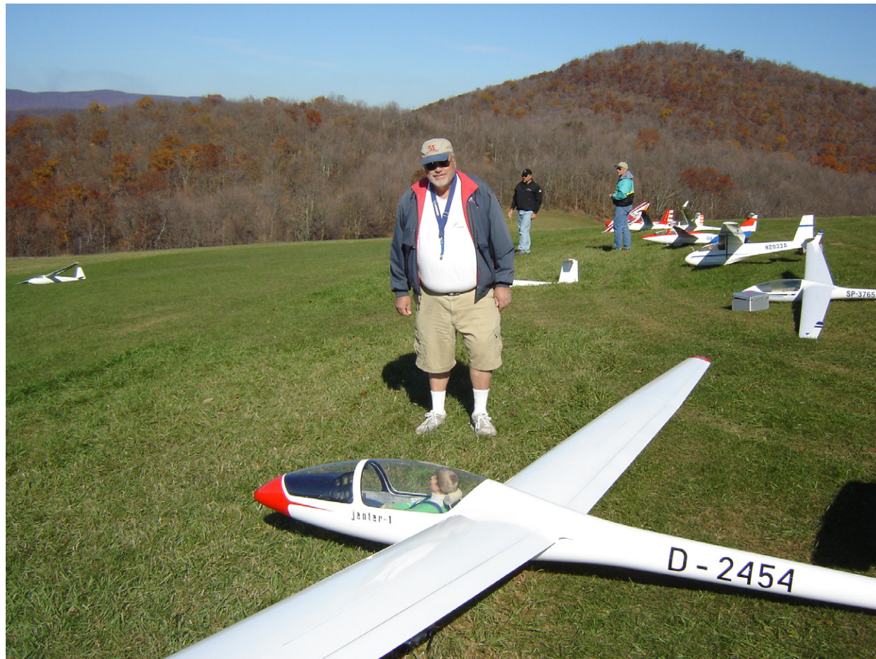
Myer Gutman is the happy pilot of this Jantar. It weighs 55 pounds and has a 26 foot wing span and thermals with the best of them.
