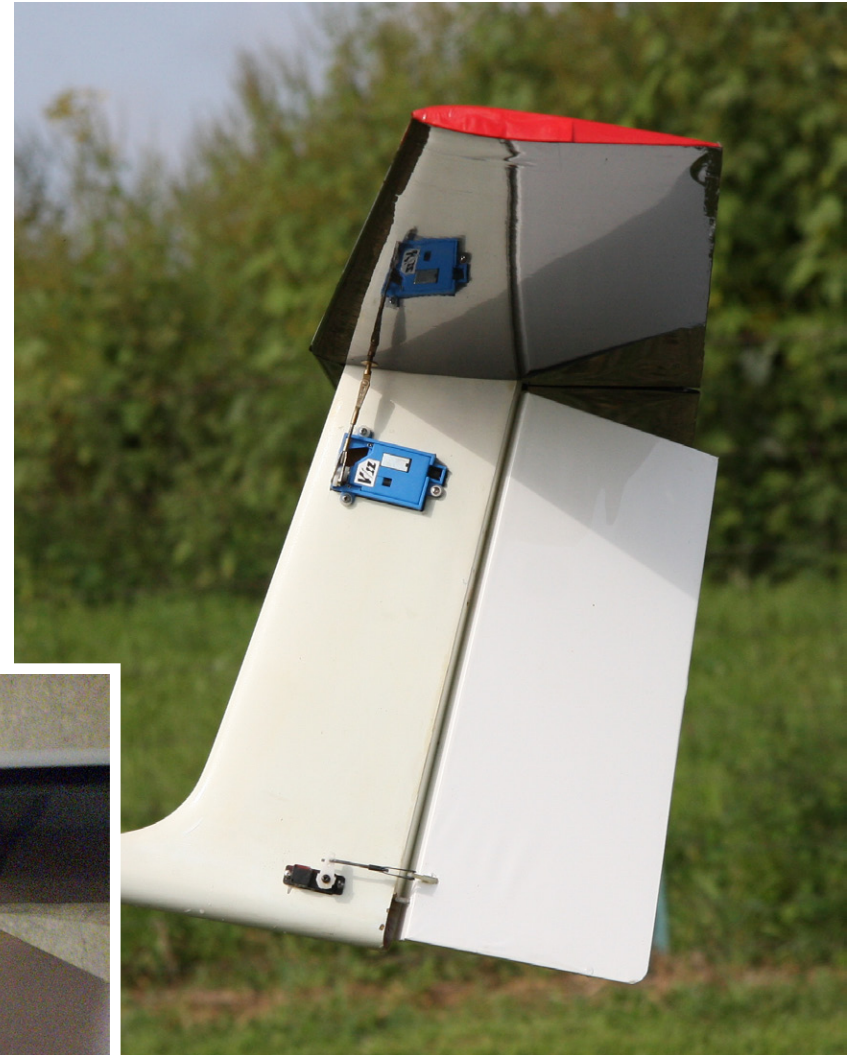
Above and left: Strong Volz metal geared digital servos in the tail for both the rudder and the stab, making them rock solid.
