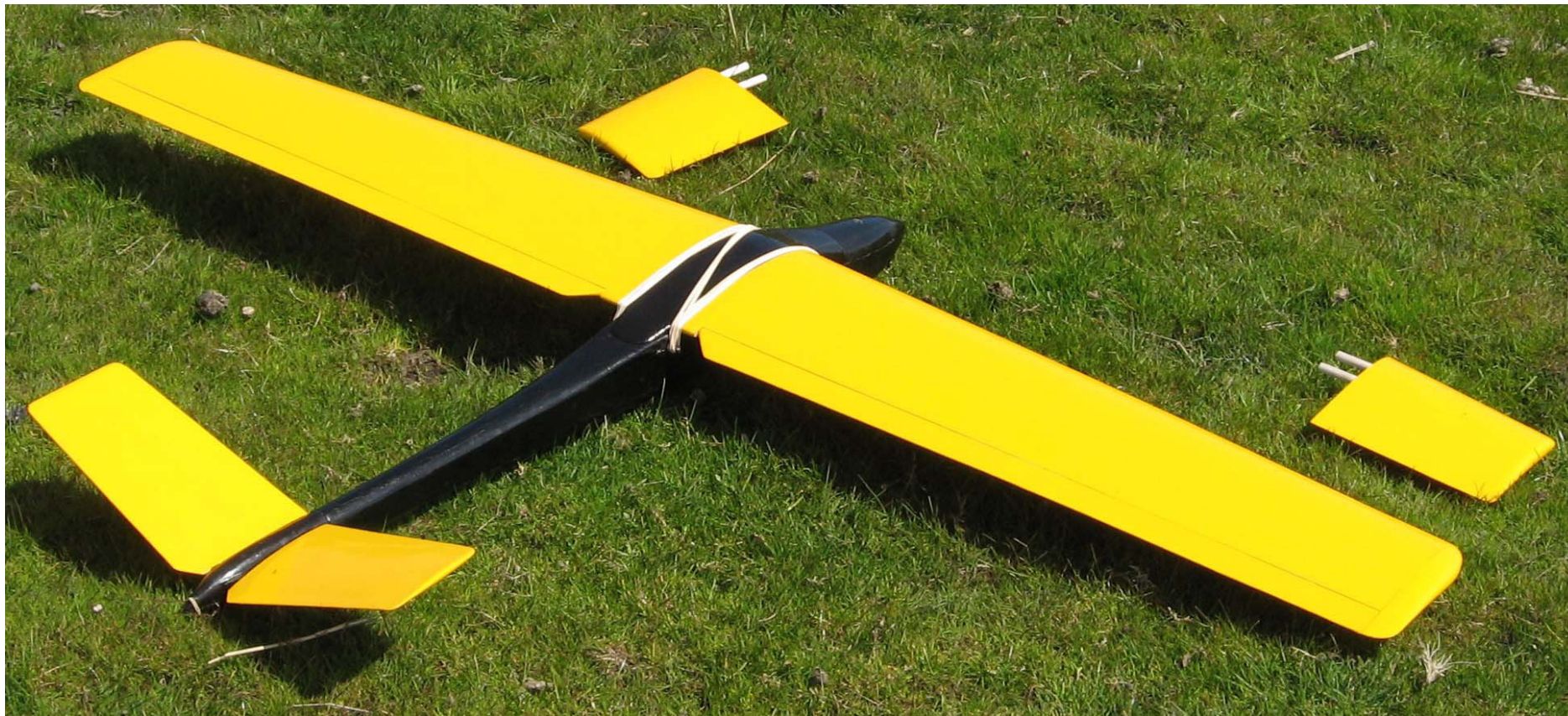
The author's model with its new wing, 66" span. The plug-in extension wing tips which are seen in the photo below are for use in weak lift.
