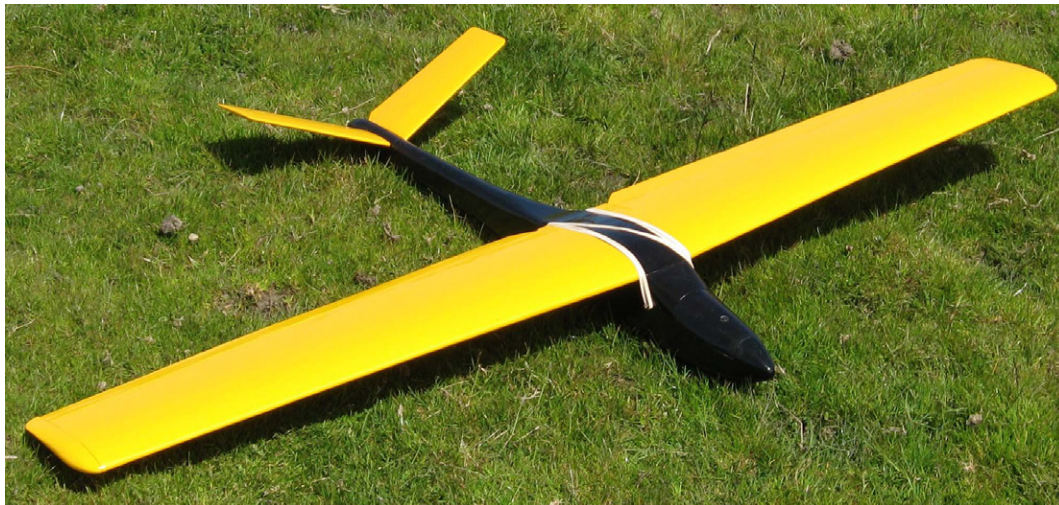
The author's model with its new wing, 66" span. The plug-in extension wing tips which are seen in the photo below are for use in weak lift.
