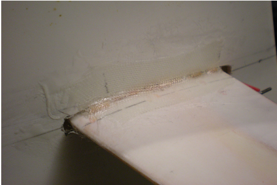
Here is the stabilizer with the 2 oz. glass securing it in place.
