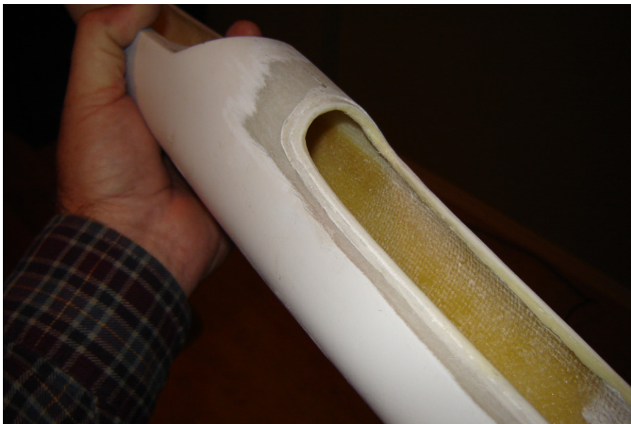
These photos show the new epoxy added to the fuselage to make a seat for the canopy.
