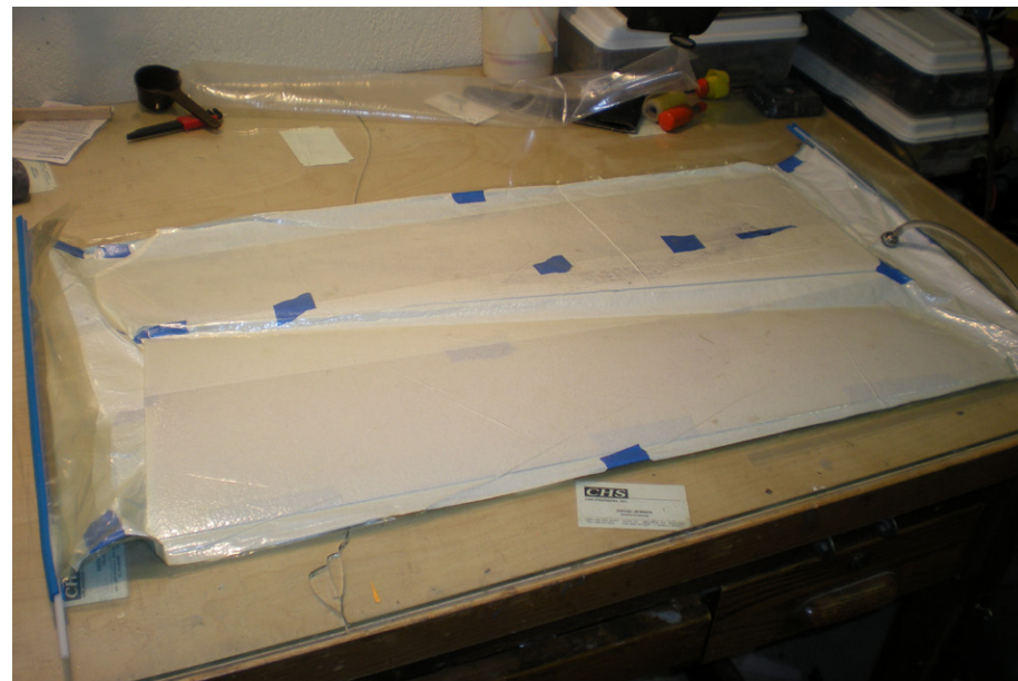
The top layer of glass being vacuum bagged.
