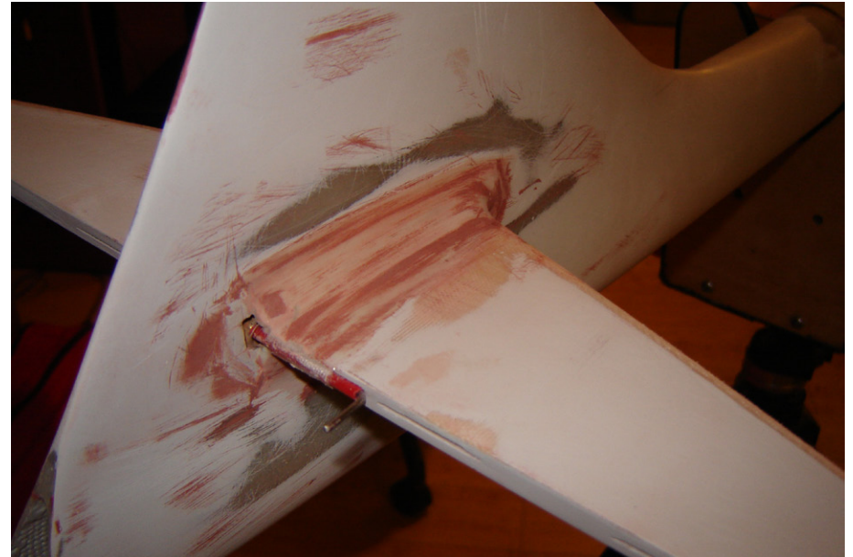
Here the epoxy fillet is sanded to rough shape.
