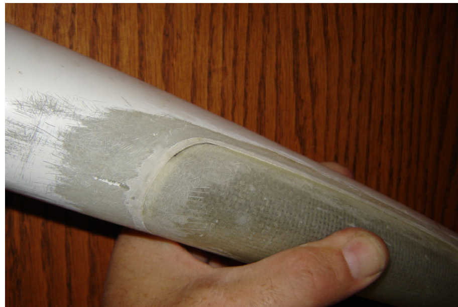
These photos show the new epoxy added to the fuselage to make a seat for the canopy.
