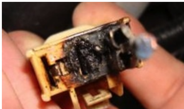
The result of a 12 Volt gremlin attack. The black charring is indicative of an arc.
