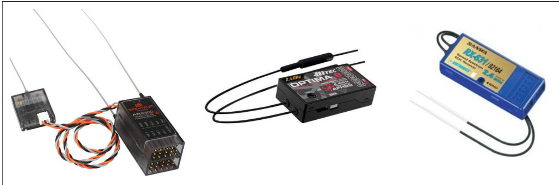
1. Contemporary 2.4 GHz receivers, all with multiple antennae. The Spektrum 9300 on the left has a satellite receiver as well.
