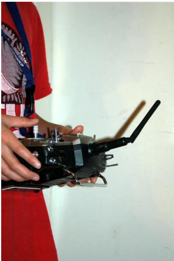
EXAMPLE 1: The most recommended angle of the Tx antenna for flying, for the average pilot who holds his Tx at this angle. This is a 45-degree bend.
