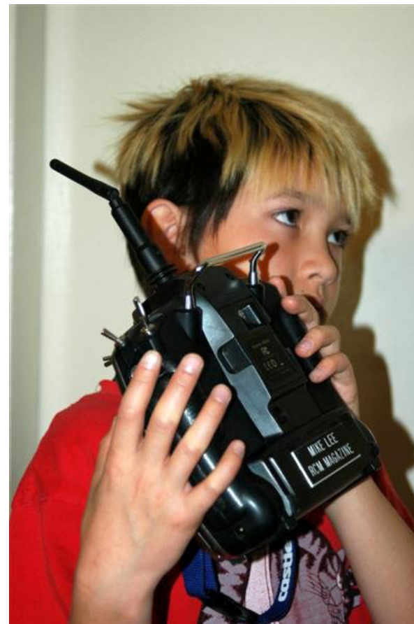
EXAMPLE 3: For those pilots who use body English, or just get animated with holding the Tx, this angle is also a no-no. It goes that like the earth, there is a polarity to the radiation pattern of an antenna. So, if there is a North Pole being at the tip of the antenna, then there is a South Pole at the bottom. Therefore, if there is a Cone of Silence at the top, there will be another one at the bottom! Want to prove this to yourself? Do some flights with a Flight Log device and you will find out!
