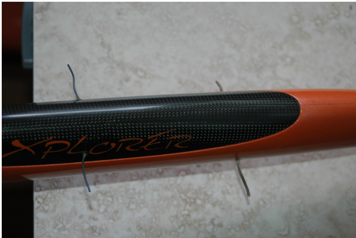
My NaN Models XPLORE with an AR7000 Rx and one remote Rx installed. Note the antenna placement... not what is recommended, but it has been flawless in operation.
