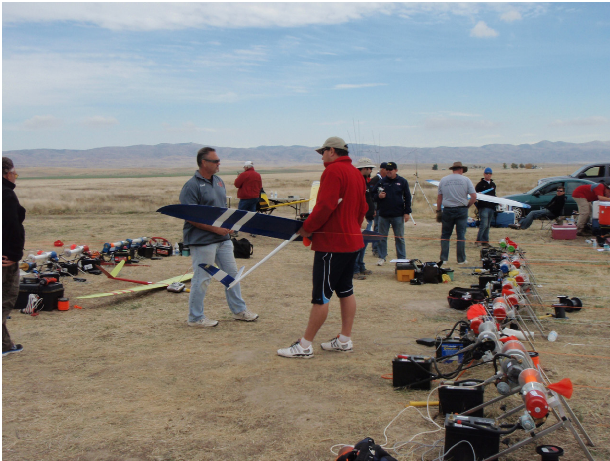
Daryl Perkins does a last minute check before flying. Note the two rows of winches, set up so that launches are always up wind.
