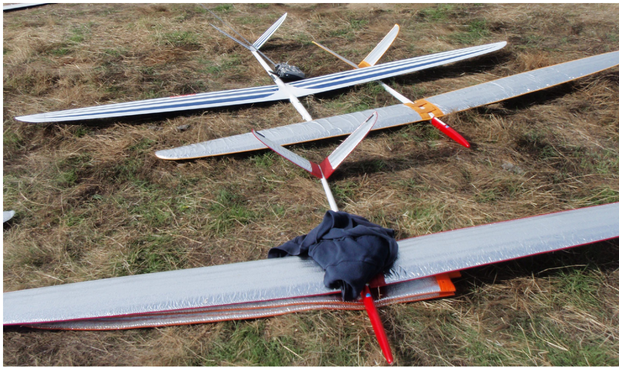
A selection of 'ships specifically designed for the three F3B tasks - Duration, Distance and Speed. Because of the relatively low weight given to landing points, V-tails are more popular here than in the usual thermal duration contest.
