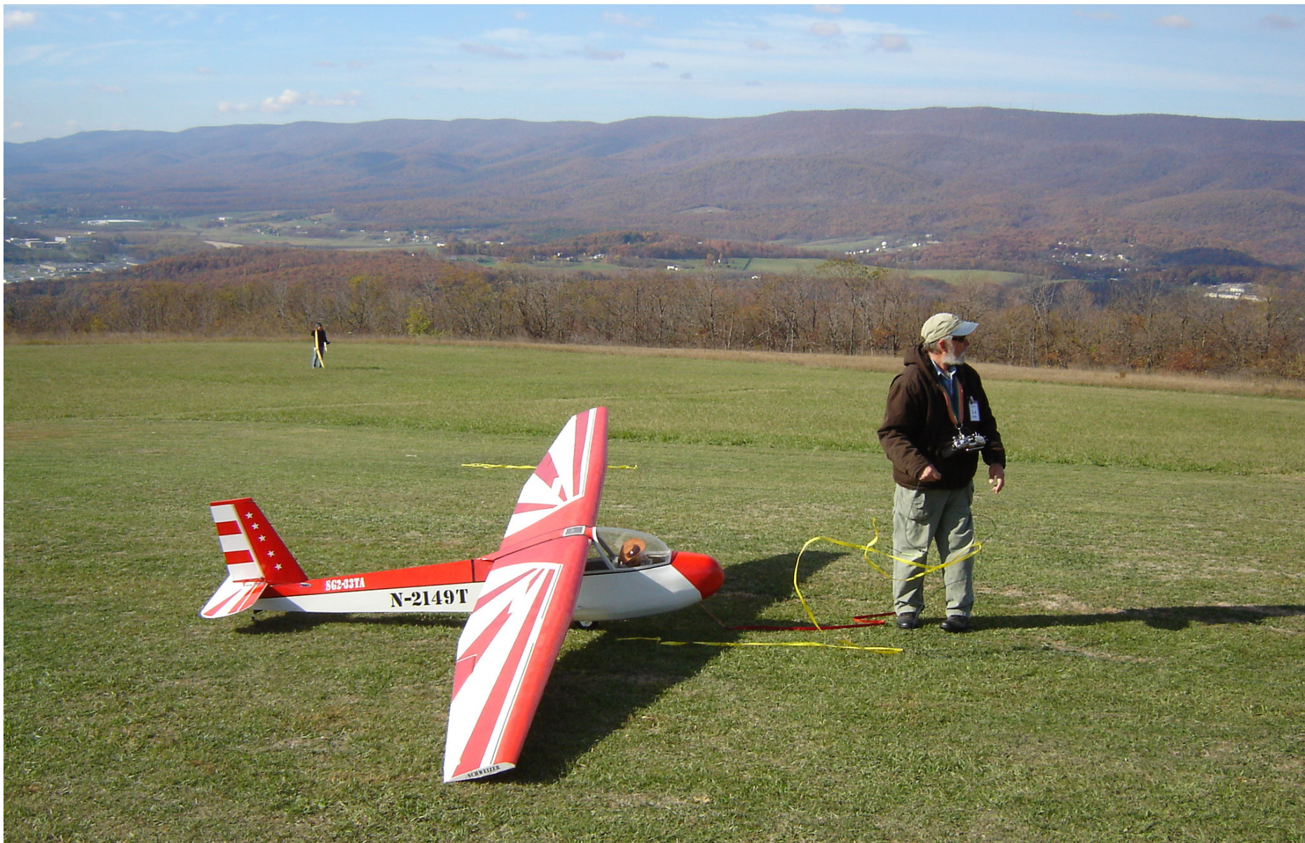
This Schweizer 2233 scale sailplane was towed to the launch area with a strap by its pilot. It was of balsa construction with Monokote covering. Its pilot figure wore a cowboy hat, which is a nice contrast to the usual white sailor hat.
