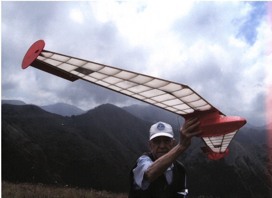
Left: Photo 1 — Nino Renzi, a real oldtimer of Genoa, has built a perfect replica of the MD-14, equipped with radio control, transforming the original external aluminum flaps into full service elevons. Thus only two servos are required.
