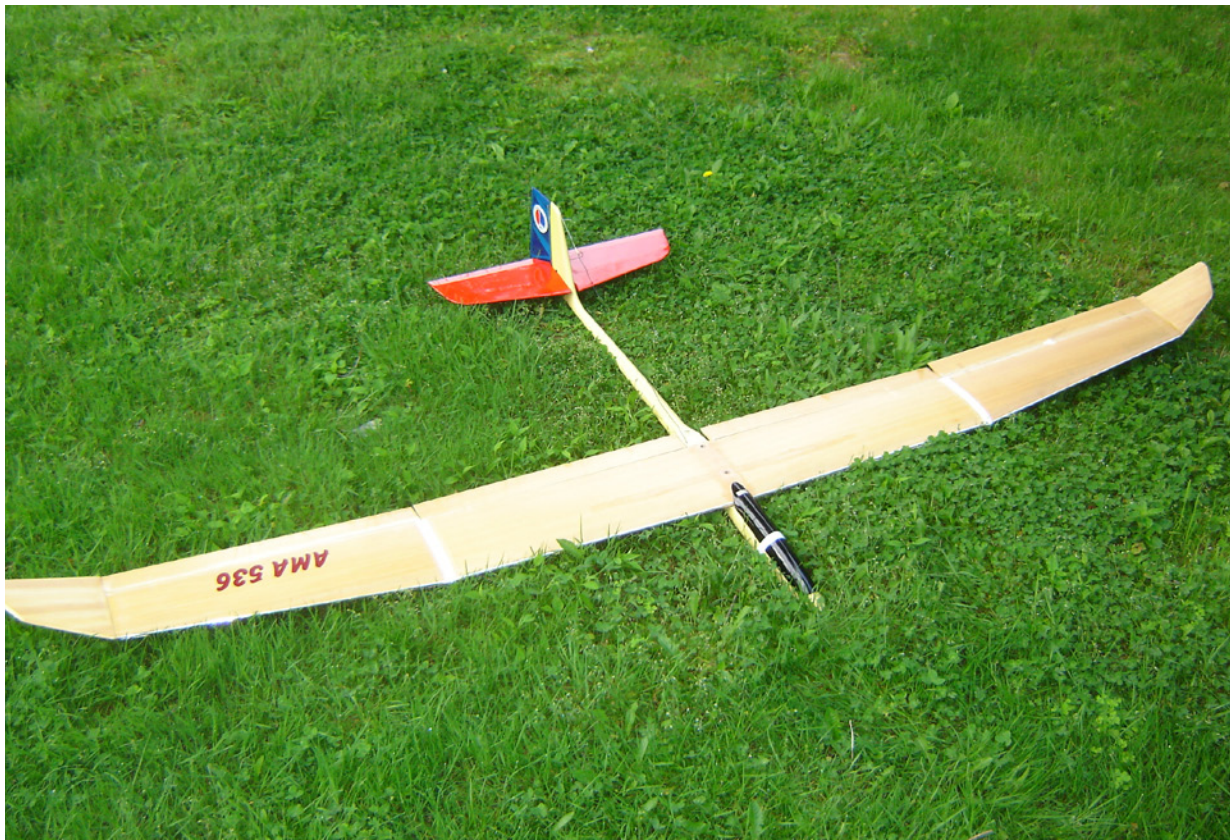
A Whyte Wings Jade with the extended wing tips. Wing loading is about 13 ounces per square foot with veneer-over-white-foam construction.
