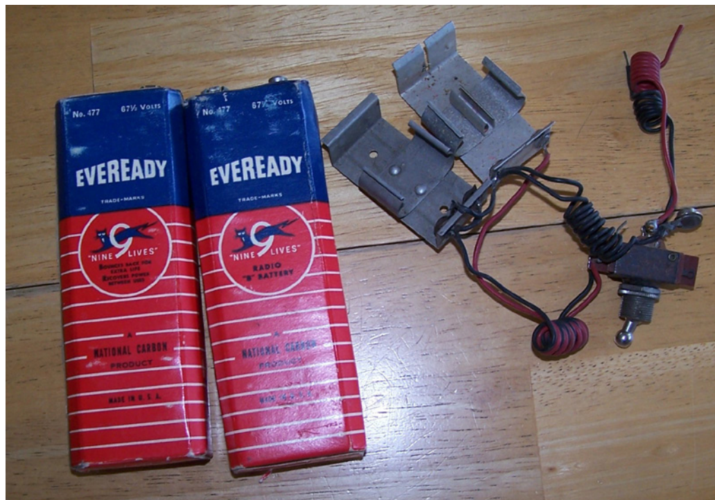
Above: Two large (nearly 6" long) 67 \frac{1}{2} Volt plate batteries on the left. The wire harness at right has two battery holders for the filament AA batteries which were changed often. Photo by Jerry Slates
