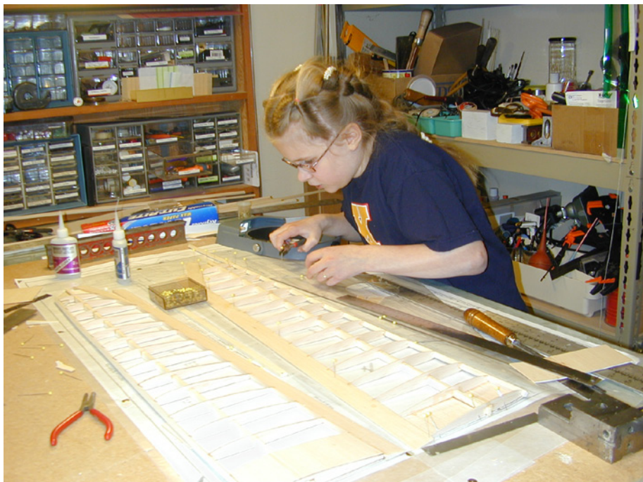
Anna pulls pins from the wing framework after the CA cures.
