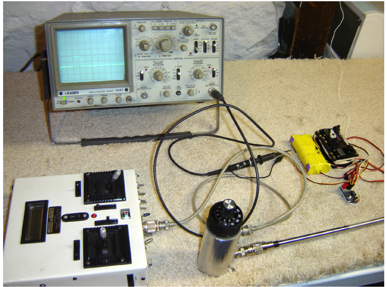
A MicroPro 2000 encoder with FMA RF deck in a ACE case comprises the transmitter at left. The SO-239 and PL-259 adaptor connectors are at the transmitter top. The Step attenuator and telescoping antenna are at right. The Leader oscilloscope displays the single channel pulse at the rear.
