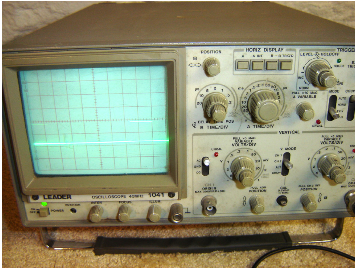
The Leader 1044 40 MHz scope displays a single decoder output pulse at 2 volts per division vertical scale. Both receivers had a about the same pulse amplitude. Noise was barely visible in this scope trace.
