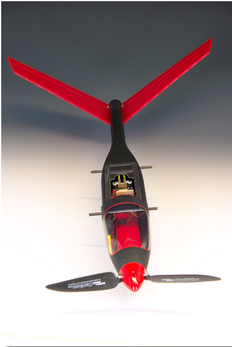
This is view of the fuselage with all parts installed and waiting for the wing.
