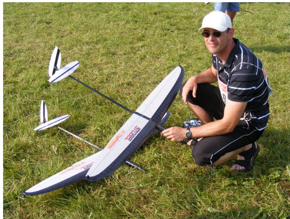
Clockwise from upper left: European molded HLG. USA Encore with vacuum bagged wing. Molded Stobel held by one of its designers, Thomas Ehrentraut. SALOnit molded carbon wing over white foam.
