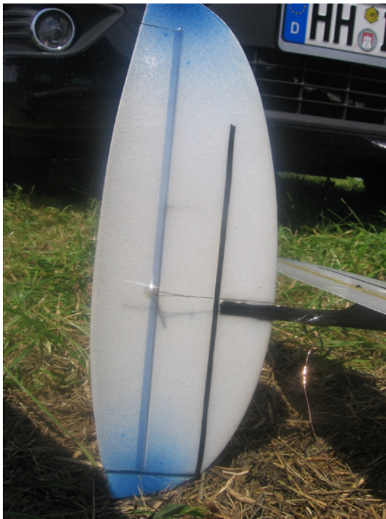
Above: Carbon fiber skinned tail group
