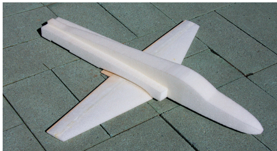
Above: Magnum Models F-5 Tiger kit contents shown after wing parts joined and spar inserted and covered with spackle. The EPP fuselage parts are shaped and joined at the factory. The balsa parts are mostly pre-cut and sanded, and the bag of small parts is shown. Not shown is the instruction manual. Below: Early construction step where the wing is completed, including installation of the aileron linkage, and now ready to begin fuselage shaping.
