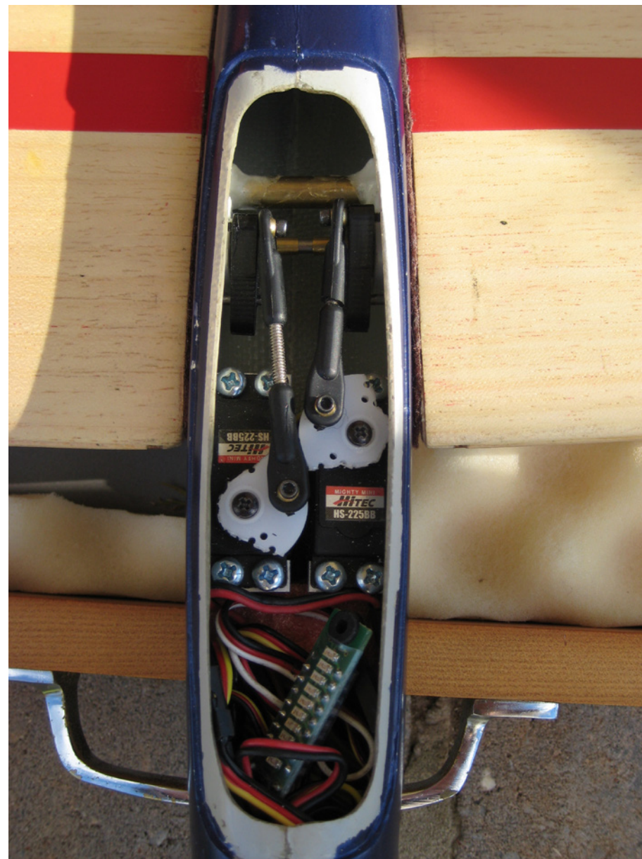
Detail of the wingeron/pitcheron system.
