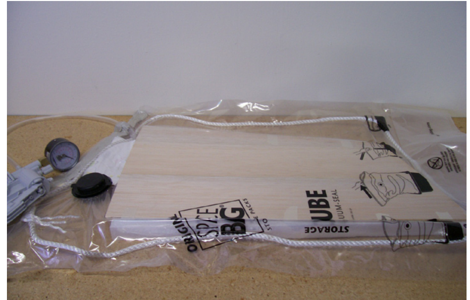
Vacuum bagging with MityVac hand held brake bleed kit.
