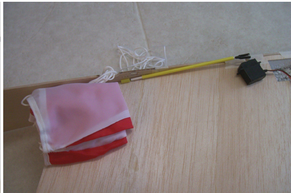
The drogue 'chute and associated servo linkage.
