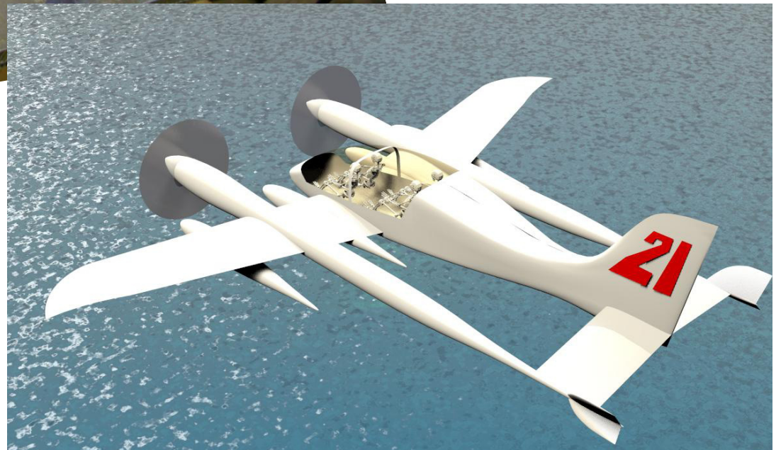
The Pond Commuter , a turbine powered play on the Pond Racer . Uses Roncz sections.
