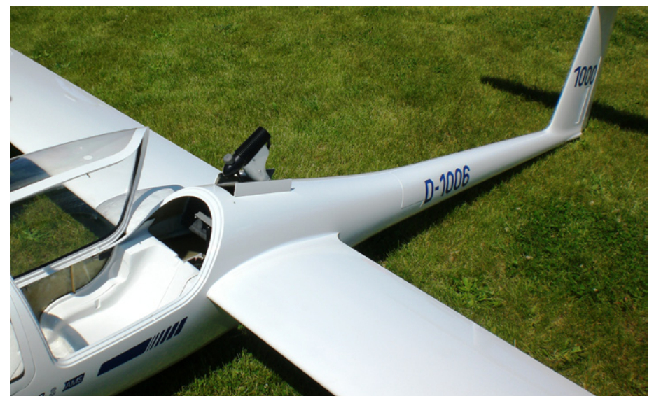
Mario Scolari's spectacular Paritech 44% DG-1000 with AFT25XS "up-and-go" unit. The single bladed prop allows for easy slide-in retraction of the power pylon through a small doored opening. Photos on opposite page by Mark Nankivil, this page by Gordy Stahl.
