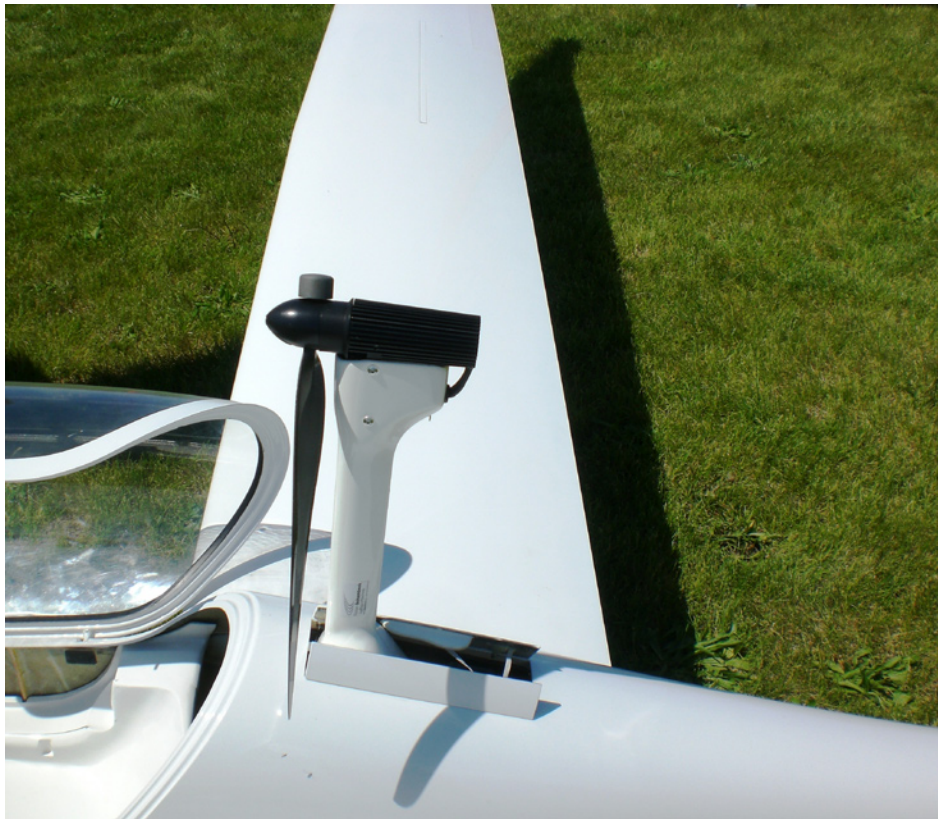
Mario Scolari's spectacular Paritech 44% DG-1000 with AFT25XS "up-and-go" unit. The single bladed prop allows for easy slide-in retraction of the power pylon through a small doored opening. Photos on opposite page by Mark Nankivil, this page by Gordy Stahl.
