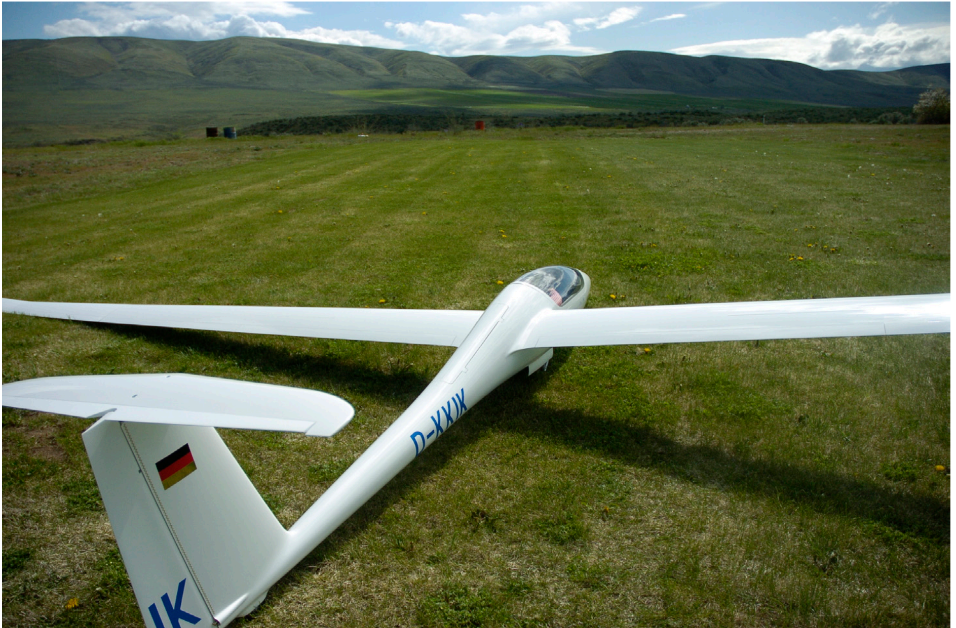
Dave Beardsley's 1/3 scale LET Ventus 2c M waits patiently to once more take to the air. The model spans six meters and utilizes a 12-channel radio system. It sports a retractable "up-and-go" electric drive with 21" prop running off a 10s LiPoly battery pack. Photo taken at the Yakima Aerotow 2006 event by Dave Beardsley. Nikon D2H, ISO 200, 1/3000 sec., 18mm, f3.5
