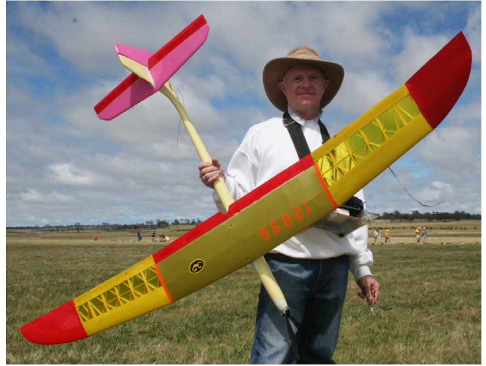
Above: Mandrella based on Ray Pike's Mantaray, 2m wing, 1kg weight, 3S LiPo, and Feigao 380-6L motor.
