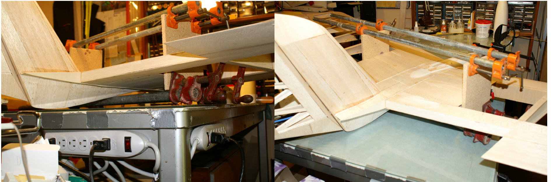
Above: Installing the lite-ply wing root caps. Pipe clamps and fiberboard leverage the wings against the fuselage center section. Below: Radio installation. A 5-cell 3300 mAh NiMH battery up front, rudder servo aft. The receiver, a Hitec RCD9600, is held in place with a large patch of Velcro. Servo wiring and rudder pushrod go down the left side of the fuselage, antenna down the right.
