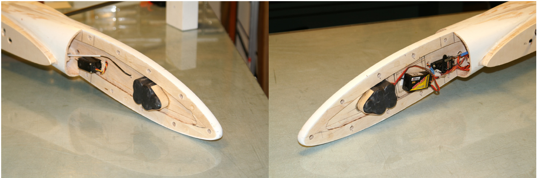
Above: Installing the lite-ply wing root caps. Pipe clamps and fiberboard leverage the wings against the fuselage center section. Below: Radio installation. A 5-cell 3300 mAh NiMH battery up front, rudder servo aft. The receiver, a Hitec RCD9600, is held in place with a large patch of Velcro. Servo wiring and rudder pushrod go down the left side of the fuselage, antenna down the right.
