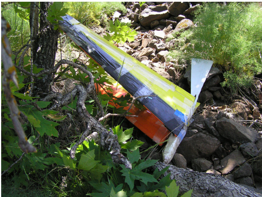
Dave's scratch-built Delta, core cut by Chris, snapped spar.
