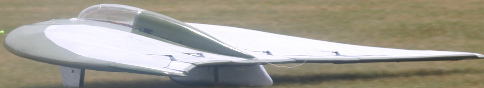
Chris Lash's Horten Parabel. Chris, from Savage Maryland, built this 'ship from foam, glass, and plywood. The Parabel is a real a heavyweight at about 50 pounds ready to fly. Futaba radio gear. As can be seen by the above photo, it did fly this year.
