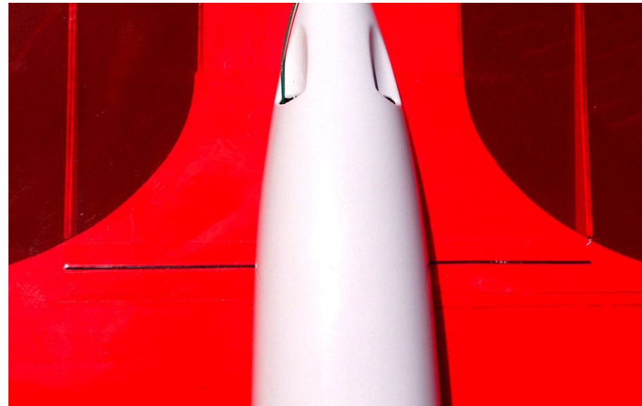
Above left: Horizontal stabilizer. Note the cutaway covering for gluing. Right: Black lines mark CG location. Note air exit holes. Below left: Thin lead strips under stab cure slight nose heaviness. Right: The front end. Folding prop, air inlet in shaded canopy
