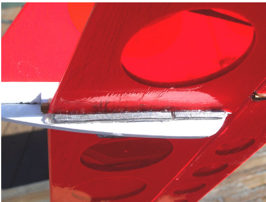
Above left: Horizontal stabilizer. Note the cutaway covering for gluing. Right: Black lines mark CG location. Note air exit holes. Below left: Thin lead strips under stab cure slight nose heaviness. Right: The front end. Folding prop, air inlet in shaded canopy
