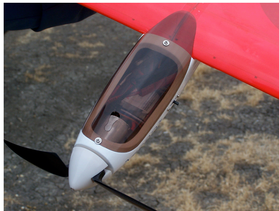
Above left: Horizontal stabilizer. Note the cutaway covering for gluing. Right: Black lines mark CG location. Note air exit holes. Below left: Thin lead strips under stab cure slight nose heaviness. Right: The front end. Folding prop, air inlet in shaded canopy
