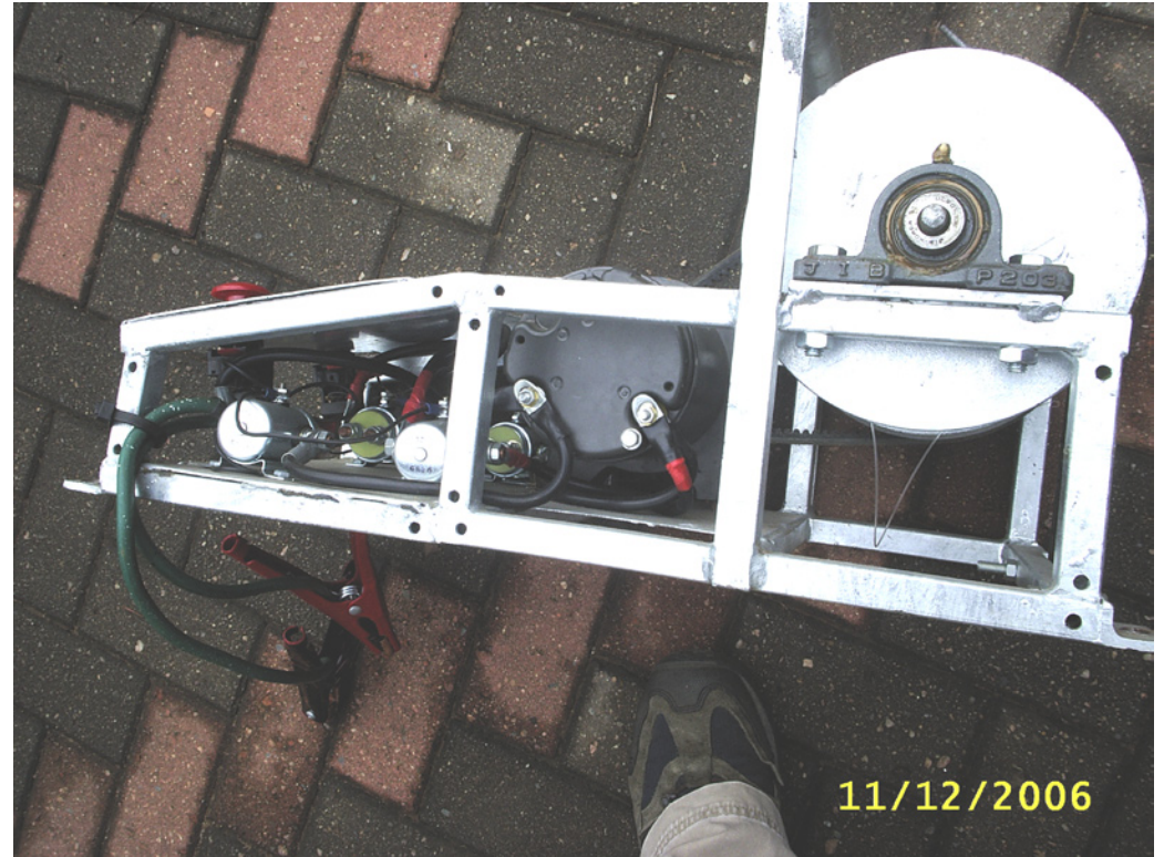
Left: Completed retriever, showing the forks (cut from an old shopping cart handle) and drum. Right: Side view of the retriever frame, showing buttons and wiring, solenoids, reversible motor and drive belt, and drum with bearings.
