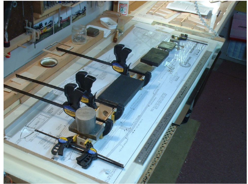
Left: Rehearsal for fuselage glue. Cut and sand where needed for correct fit. Right: Final fuselage glue with weights and clamps. Tail was glued together first as indicated in plans, then sides were warped around fuse bottom.
