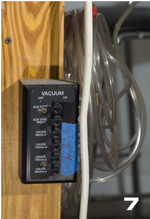
Photo 7: Vacuum manifold with toggle actuated valves that turn the vacuum on and off to the plastic hoses coiled on a hook in the right of photo.
