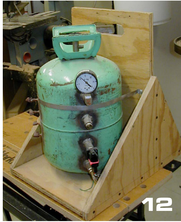
Photo 11: My first vacuum system, which was built around for about $30. The carrier was cut from a plywood shipping crate.
