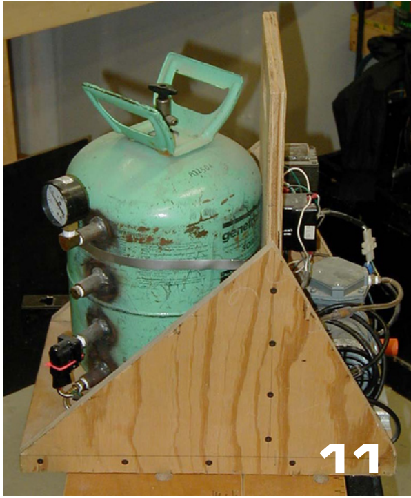
Photo 11: My first vacuum system, which was built around for about $30. The carrier was cut from a plywood shipping crate.
