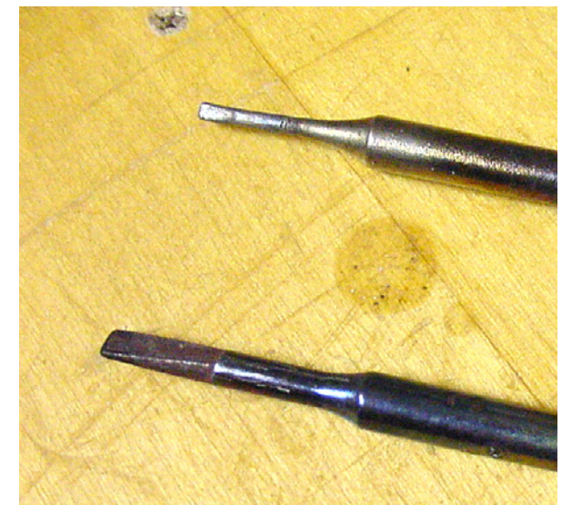
Small and large soldering iron tips. Both of these examples have chisel-shaped ends.
