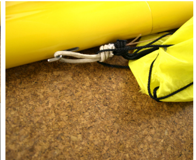
Pass line through 'chute cord and secure as shown above.
