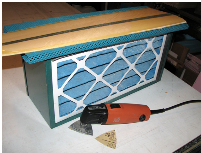
Left: Close-up showing leading edge trimming. Scissors are sometimes sold for trimming plastic kit parts. Right: Remaining flash is trimmed with a Fein sander and 80-grit aluminum oxide sandpaper. 20,000 orbits per minute allow rapid removal of the remaining flashing. Dust is captured with a bench-top filter from Grizzly.com.
