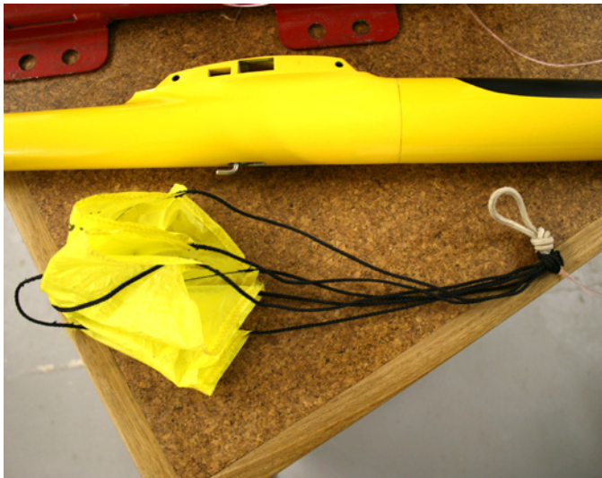
Arrange the 'chute cord to create a loop.
