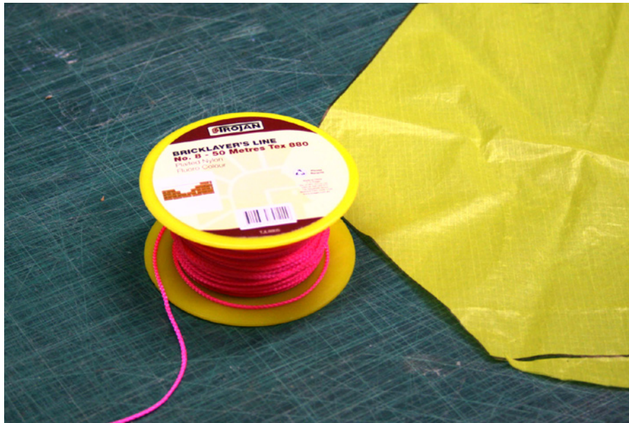
#8 bricklayer line is used for the parachute lines.
