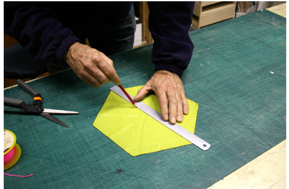
Use pencil lines to assist in laying-out the cord.
