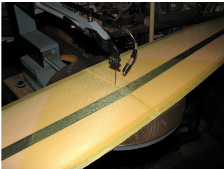
Left: After the mylars have been removed from the vacuumed-bag wing the wing is cut into two pieces with a fine-toothed jig saw. Right: Excess leading edge flashing is first trimmed with curved lexan-trimming scissors and sharp side cutters. Shelf liner material is placed under the wing to minimize denting of the surface.
