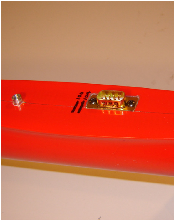
Left: The DB9 connector mounted to the fuselage. There's a matching depression in the bottom of the wing. Right: Under the canopy of the Xperience Pro-X interior; from left — Hitec Super-Slim receiver, switch, battery monitor, rudder servo, elevator servo.
