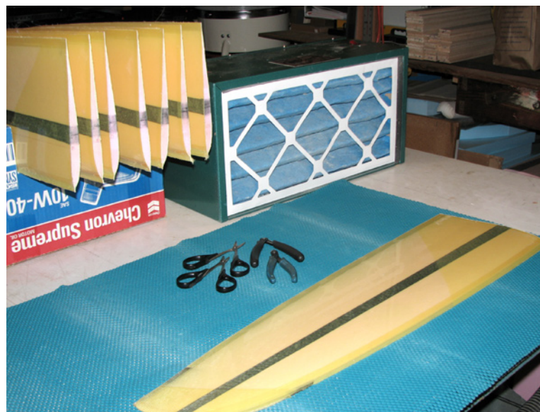
Left: After the mylars have been removed from the vacuumed-bag wing the wing is cut into two pieces with a fine-toothed jig saw. Right: Excess leading edge flashing is first trimmed with curved lexan-trimming scissors and sharp side cutters. Shelf liner material is placed under the wing to minimize denting of the surface.
