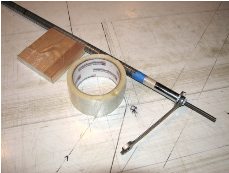
Left: Cured boom ready to be removed from mandrel. 1/4" rod epoxied in ski pole and nuts jammed on for wrench to allow twisting of mandrel in tube to facilitate release. Wood clamp taped to shrink-wrapped carbon tube. Right: Another view of the clamp. This is a very effective way to hold the tube while twisting and pulling the wrench/mandrel during release process.
