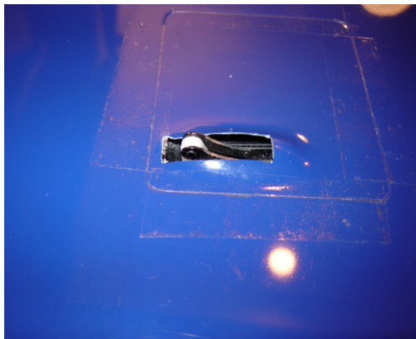
Flap servo well and cover. Note trimmed lip. New servo covers will be fabricated.
