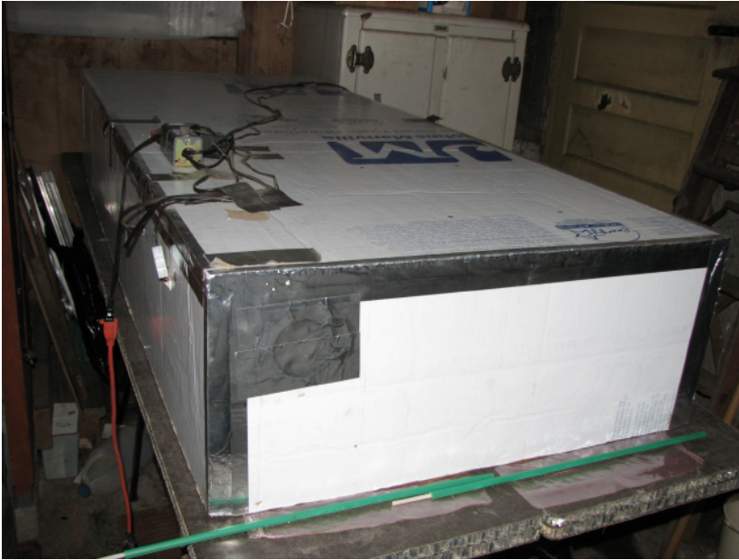
Above: The exterior of the heat box. Two wings are usually cured at once.
