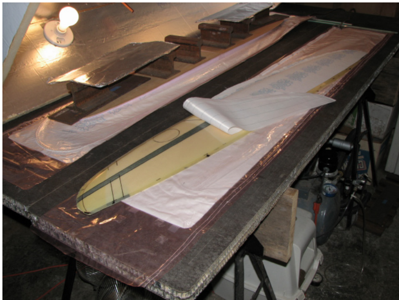
Left: Upper breather/peel ply layer removed from the mylar/core sandwich. The lower breather-peel-ply layer remains in the bag. Right: The tape holding the mylars together is cut and the mylars peeled back revealing the shiny surface of a new wing.
