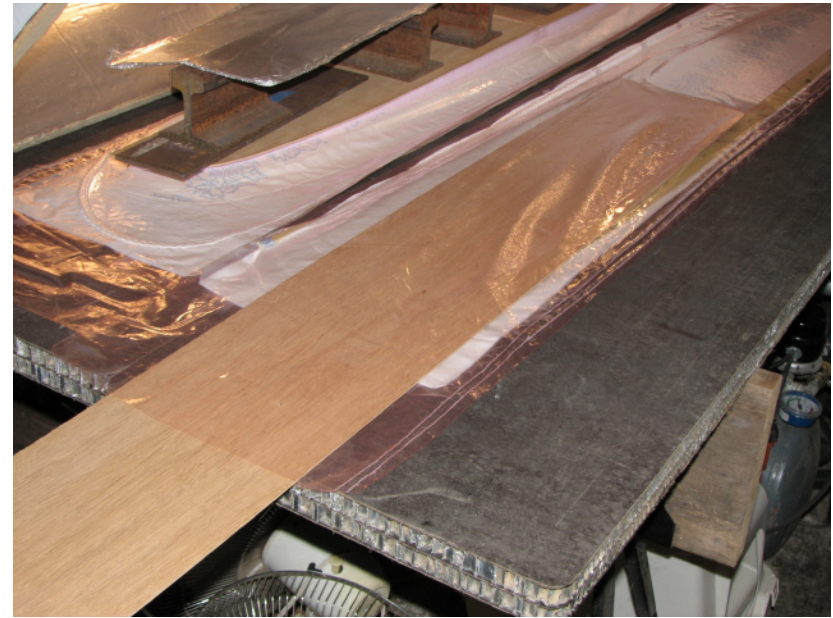
Left: Vacuum is released after curing by removal of the tube locks. Right: The same plywood door skin panel used to slide the wing/ mylar layup into the bag is used to free the sticking bag from the layup after cure prior to removal of the wing.
